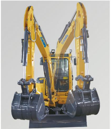
The left and right boom swing angle is respectively 75° and 50°, it can realize complex operation together with upper structure slewing to ensure that the digging is parallel with wall surface in narrow space through the cooperation of upper structure slewing so as to easily deal with various operating conditions.
